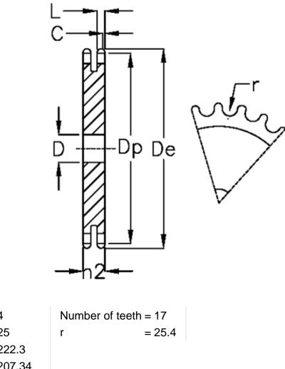
C = 4 D = 25 De = 222.3 Dp = 207.34 For chain size = 1  $1/2 \times 1$ For chain type = 24 B-2 h2 = 72 L = 23.6
